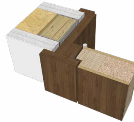
Drywall outside flush jamb with in-swing door
