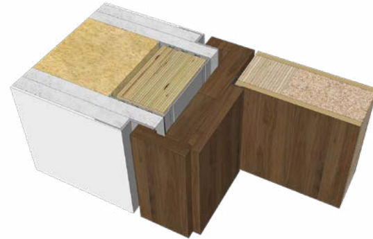
Drywall wall with shadow gap feature + Single rabbet jamb with 1 side adjustable casing
