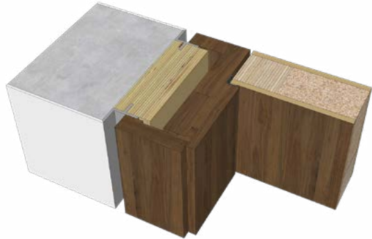
Concrete wall with shadow gap feature + Single rabbet jamb with 1 side adjustable casing
